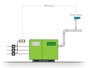
Compressor efficiency is indicated by a typical Key Performance Indicator (KPI) with units of kW/m3n/min or kW/100 SCFM.
